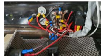
UNCOVERED - Switch, wiring and relays
