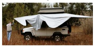
Both webbing straps must be tightened so that the awning is tight
